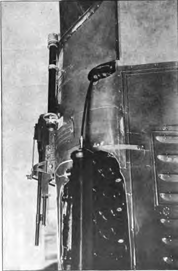
Fig. 23.—FIXED MOUNT FOR ONE MARLIN AIRCRAFT MACHINE GUN ON CURTIS-JN4-HG, SHOWING UNIT SIGHT, AUXILIARY SIGHT, AND MECHANICAL SYNCHRONIZING GEAR, TYPE H-S.
