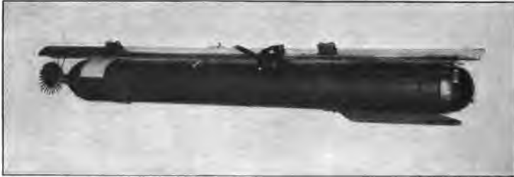
FIG. 52.—AIRPLANE FLARE, MARK-I AND RELEASE MECHANISM.
