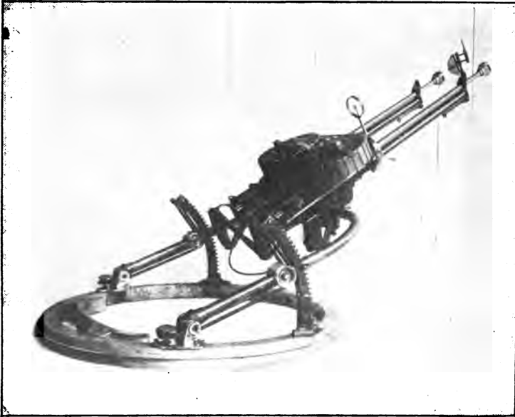
FIG. 27.—DOUBLE LEWIS GUN YOKE WITH GUNS.
