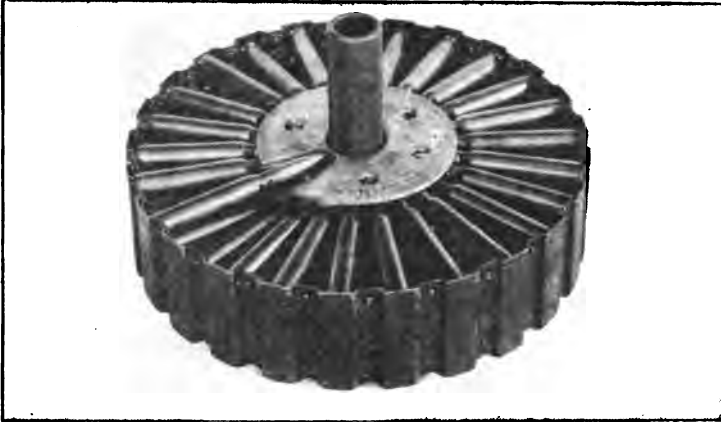
FIG. 7.—97 ROUND LEWIS MAGAZINE WITH LOADING HANDLE.
