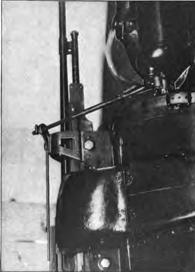
FIG. 30.—MECHANICAL SYNCHRONIZING GEAR, TYPE H-8, AS MOUNTED ON CURTISS JN-4-HG.
